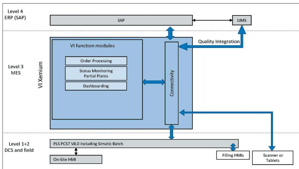
Opcenter Execution Process acts as an information hub between the ERP software and the process automation system. It also communicates with the laboratory information management system and with hand-held wireless devices for sampling, materials tracking and packaging.
