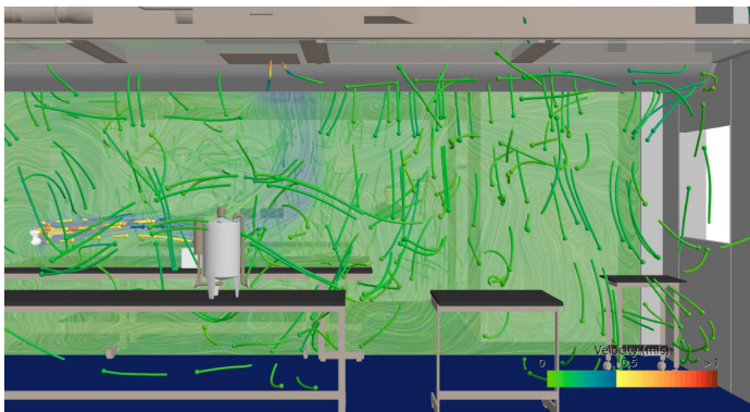
Figures 3a and 3b. Set up from scratch within a few hours, these simulations come with easily comprehensible graphic representations of particle clouds or temperature and pressure distributions.
